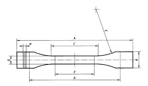
Figure 1 — Test piece obtained by machining (type 1)
