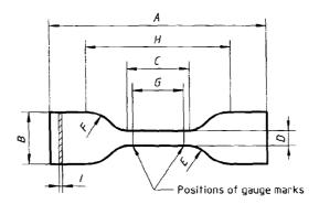
Figure 2 — Test piece obtained by die cutting (type 2)
